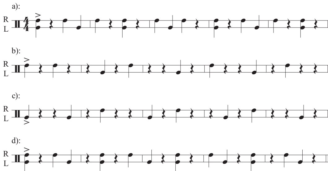
Figure 6: The pulse response of the stereo time delay effect. a): simultaneous input pulse on both channels (accented note on beat 1 in 4/4 meter), in-channel feedback. b): right channel pulse input, cross-channel feedback, c): left channel pulse input, cross-channel feedback, b): simultaneous pulse input on both channels, cross-channel feedback.
